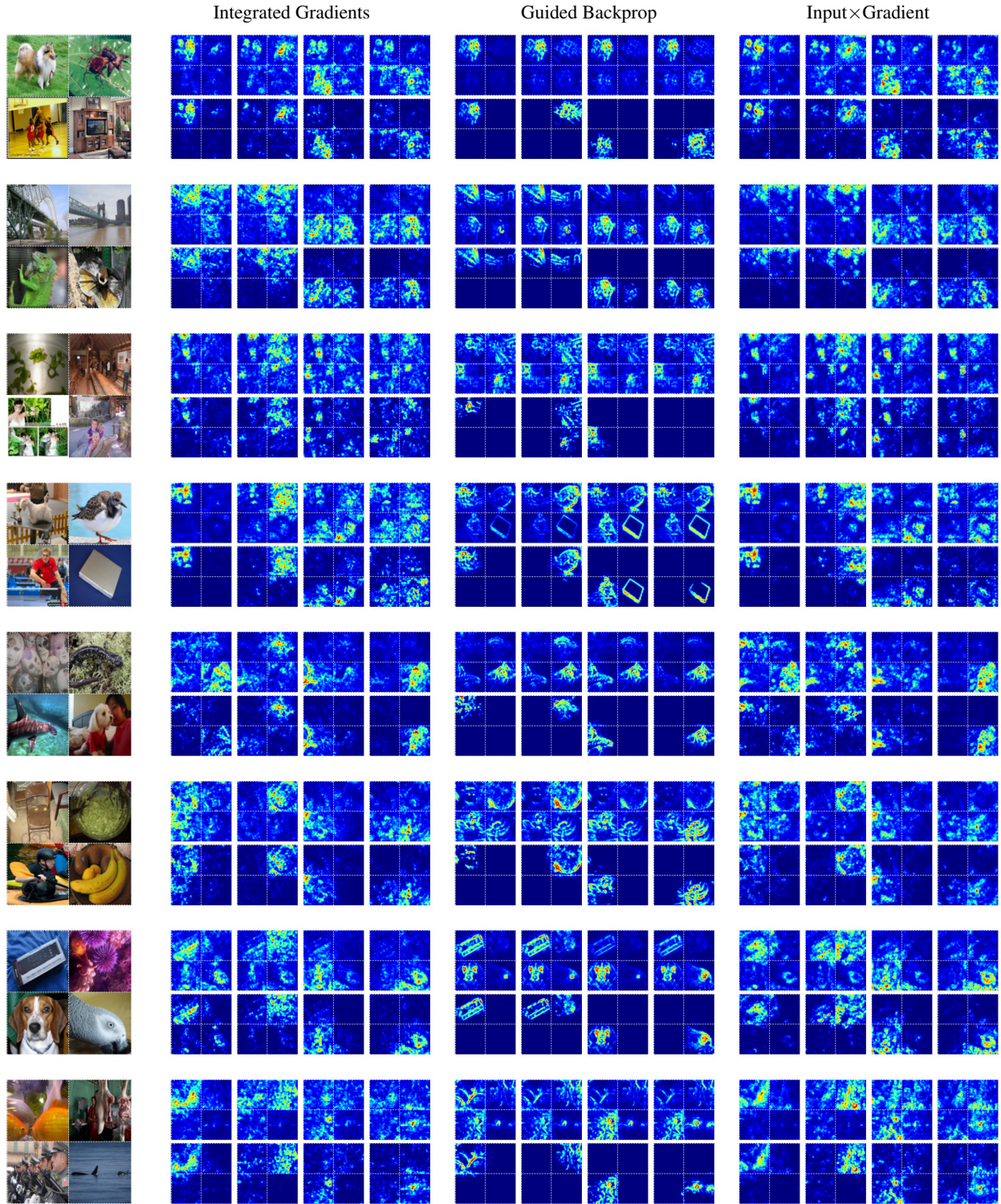
Figure 13. ResNet50 : VAR on the Grid Pointing Game. We show examples from the grid pointing game for methods most affected by our framework (as columns: Integrated Gradient, Guided Backpropagation, Input \times Gradient). Input Images are given on the left, for each we provide vanilla attribution methods (top row) and augmented with VAR (bottom row). For each, we show the attribution for the four different classes in the grid as columns.
