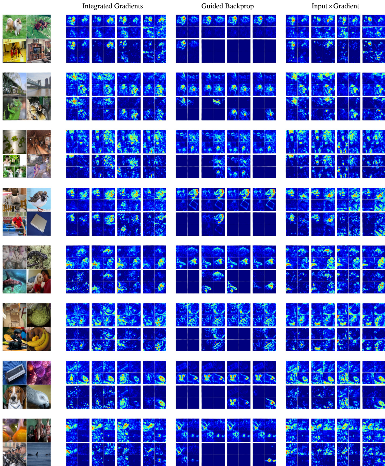
Figure 16. VGG16: VAR on the Grid Pointing Game. We show examples from the grid pointing game for methods most affected by our framework (as columns: Integrated Gradient, Guided Backpropagation, Input \times Gradient). Input Images are given on the left, for each we provide vanilla attribution methods (top row) and augmented with VAR (bottom row). For each, we show the attribution for the four different classes in the grid as columns.
